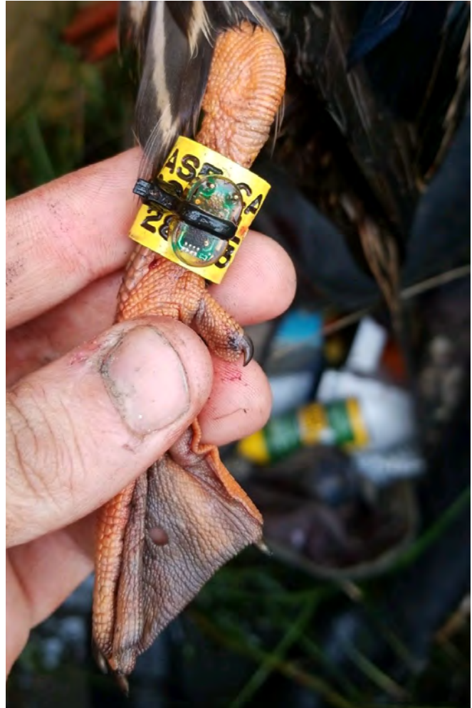
Geolocators can be used to gather breeding propensity rates but require recapture or indirect harvest to retrieve stored data.
